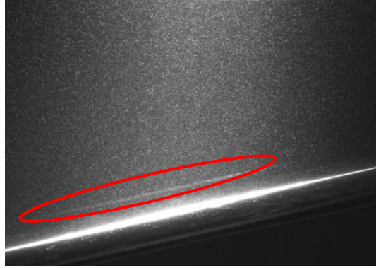
Fig. 12. PIV image showing the reflection of the light sheet (circled).
